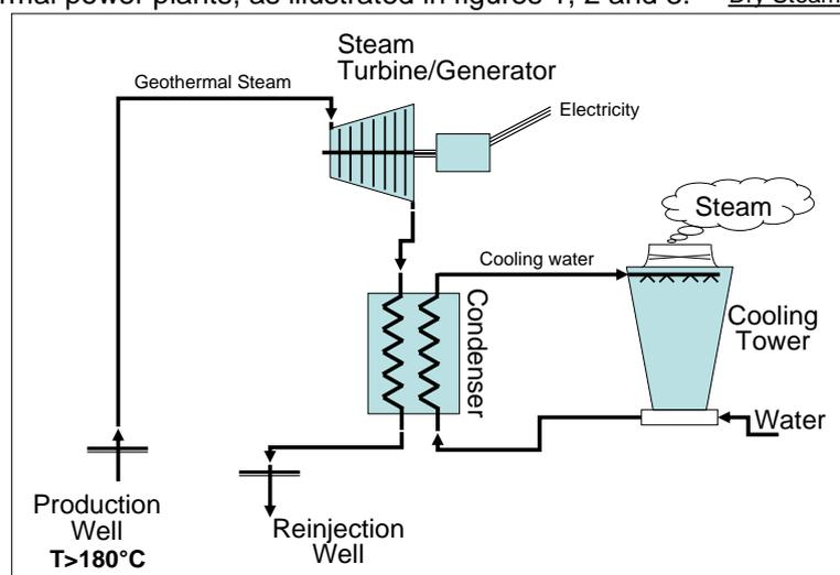
Figure 2. **Flash steam power plants** are the most common type. They use geothermal reservoirs of water with temperatures greater than 180°C. This very hot and compressed water flows up through wells in the ground. As it flows upward, the pressure decreases and some of the hot water boils into steam. The steam is then separated from the water and used to power an on-surface turbine/generator.
