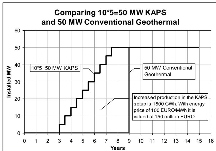
9. With the DPG model, boreholes can be harnessed at an earlier stage or within weeks after drilling is completed, whereas the CMG model requires borehole evaluation and powerhouse construction for a period of 6-7 years before commencing power production. In cases of high market prices of electricity, the increased production of the DPG approach could even pay for the total cost of the on-surface equipment of the KAPS-units. See figure 3.
