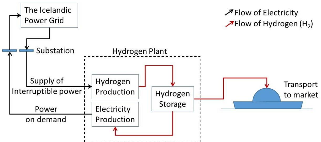
In this study we assume that the production of hydrogen is based on electrolysis. The largest financial factor of the Hydrogen Plant is price and supply of electricity. The main purpose here is to clarify the exchanges of electricity with the Grid.
